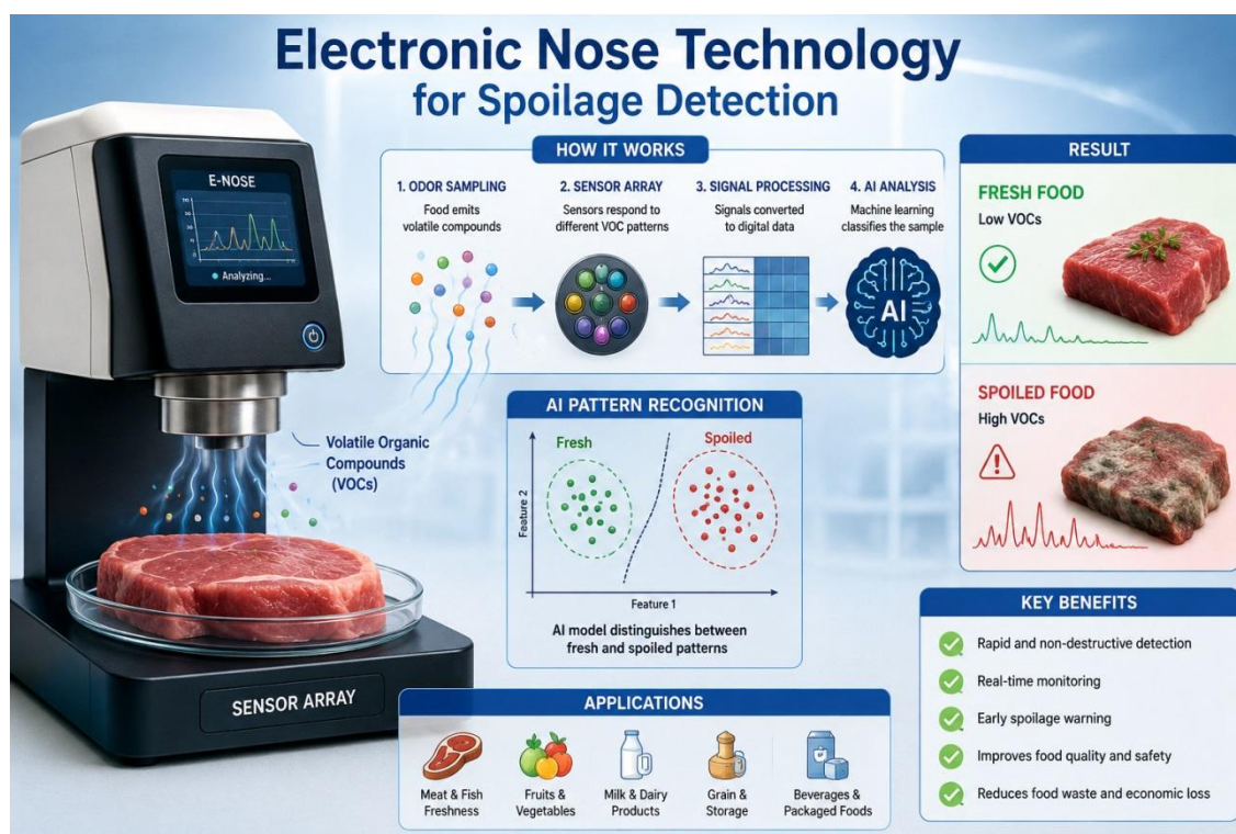
Figure 2: working principle of Electronic Nose Technology for Spoilage Detection
