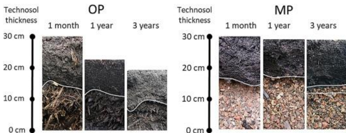
Figure 1. Technosol profiles after 1 month, 1 year, and 3 years for OP (left) and MP (right) treatment (Grard et al. , 2025)
