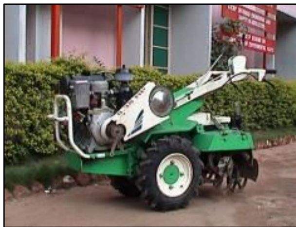
Fig. 5 Rotary power weeder developed by TNAU
